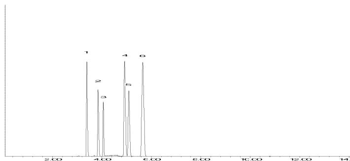
This chromatogram represents a general set of testing conditions chosen for product acceptance. For optimal results in your lab, conditions should be adjusted for your specific instrument, method, and application.
