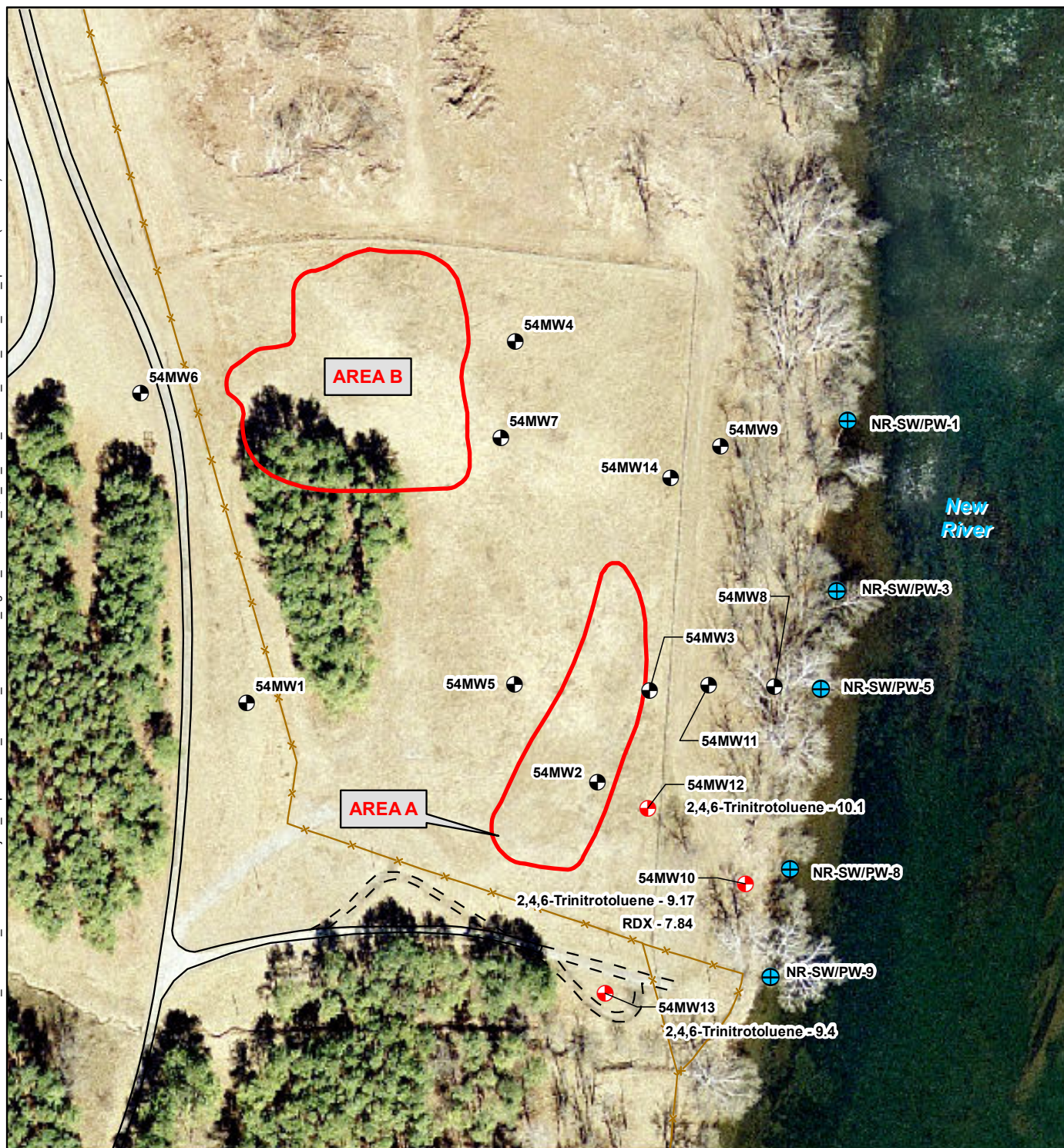
FIGURE 5-1 SWMU 54 August 2012 Groundwater Sample Results Radford Army Ammunition Plant, Radford, VA
